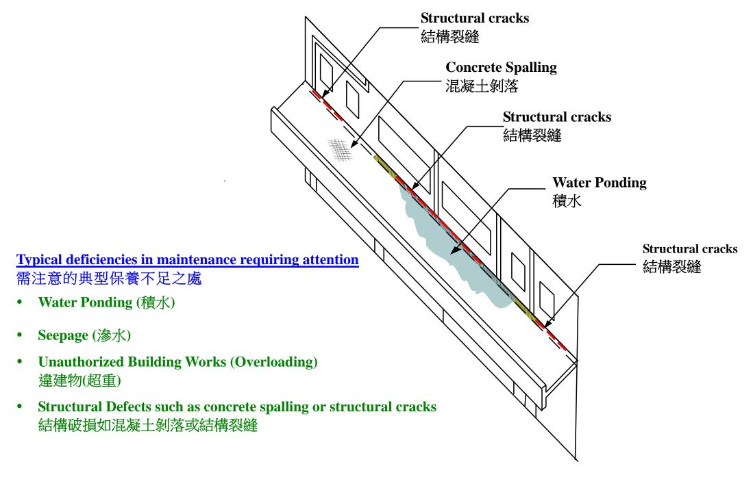
Typical deficiencies in maintenance requiring attention for Cantilevered Slab Canopy
