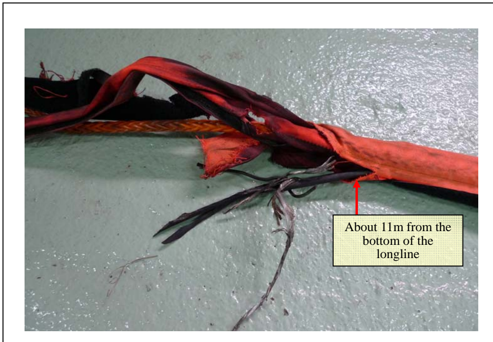
Figure 1 : The lower 11 metres of the longline's protective nylon jacket was found to have been crisped and fragmented with a large portion of the shrouded electrical cable missing.
