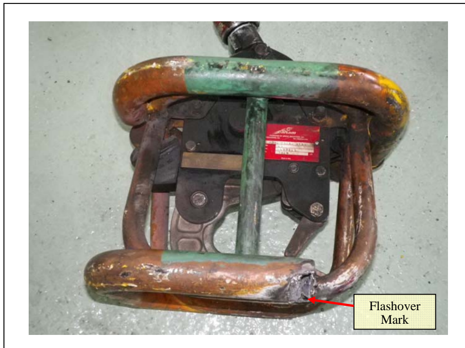
Figure 2 : The remote-controlled hook which was connected to the bottom end of the longline was charred, showing clear burn marks and signs of flashover.
