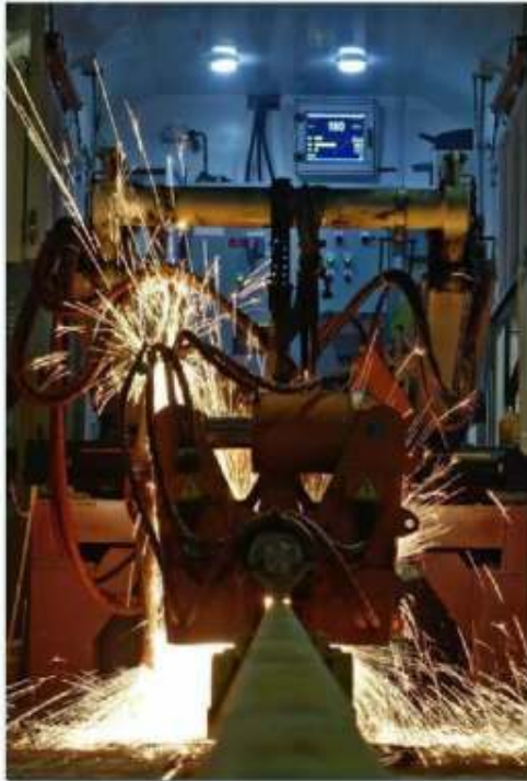
於路軌進行閃光電桿 Flash Butt Welding for Rails
