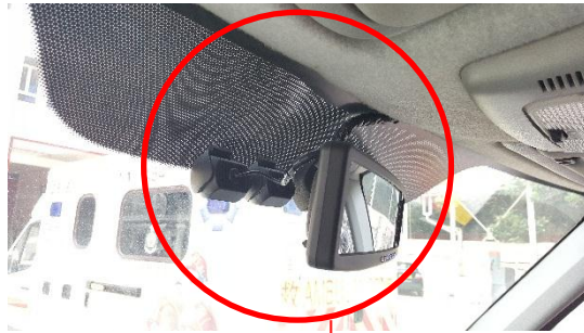
Front-view cameras and mainframe
