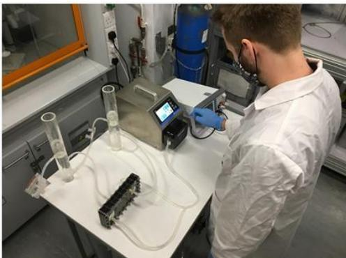
Test rig for assessing the performance of a prototype active flow membraneless electrolyzer (AFME).
